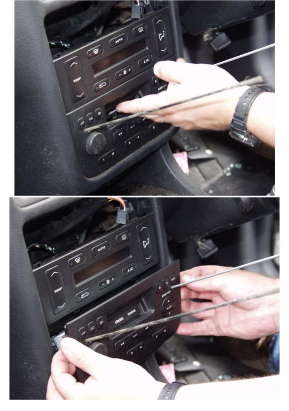
7. To remove the fascia off of the stereo unit, unscrew the small phillips/cross head screws at each end of the fascia (2 each end).
