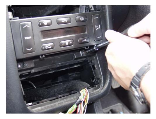
10. There are locking lugs on each side of the aircon fascia. Gently unclip these and the fascia will lift free.
