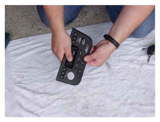
4. The smaller buttons and the "audio" sign are held on with small hooks. Use the tip of a skewer to dislodge them and push then through.
