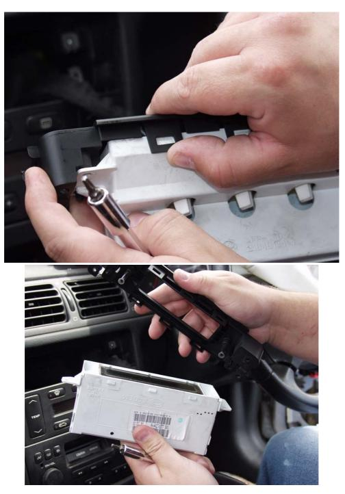
6. Gently insert skewers into the 2 holes on the fascia of the stereo unit. They should be pushed around 3 inches inward. You will then be able to gently pull the unit out. I put my finger into the cassette aperture to initialy pull it out enough to get a grip of each side. It is not paricularly stiff and should come out with ease.
