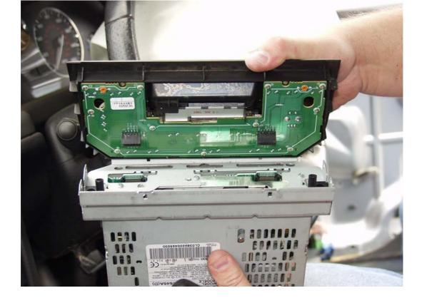
9. With the stereo unit out of the way, you gain access to the lower screws that hold the aircon unit in place. Remove these.
