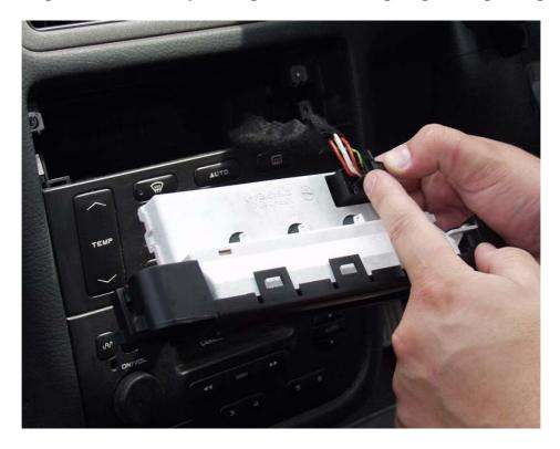
4. There is a torx screw at either end of the rear of the MFD, remove these.
