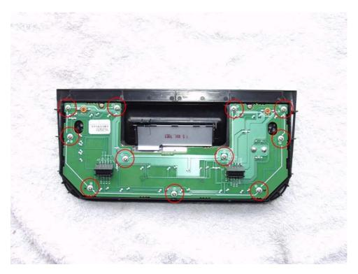
2. Now unscrew the remaing screws, also circled here for reference. This releases the clear plastic light diffuser.
