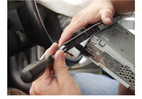
8. Gently apply pressure to the top of the fascia and one of the locking lugs while at the same time pulling slightly away from the stereo unit.
